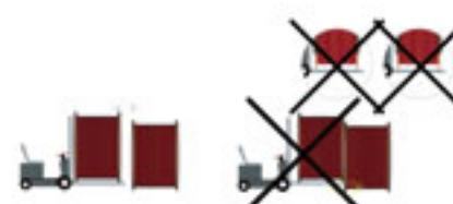
The forks must be longer than the width of the spool being lifted. Raise the forks of the forklift at least 6 to 8 inches above ground.
